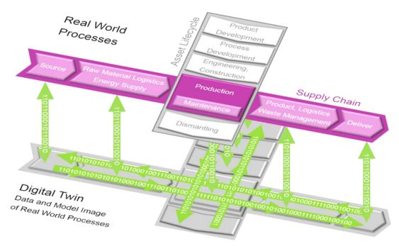
**Abbildung 1:** Schematic illustration of the digital twin as an image of the value chains of the real process world, i.e. the horizontal supply chain and the vertical asset life cycle (Source: Bröcker, Evonik)
