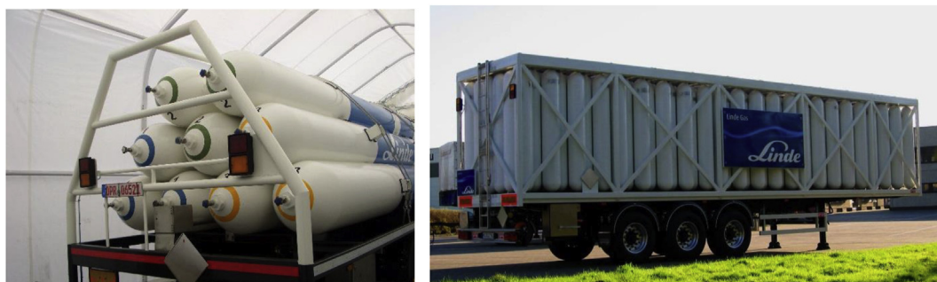
Fig. 11 – Conventional steel-tube trailer (left) and battery vehicle with 200 CPVs for hydrogen (right).
