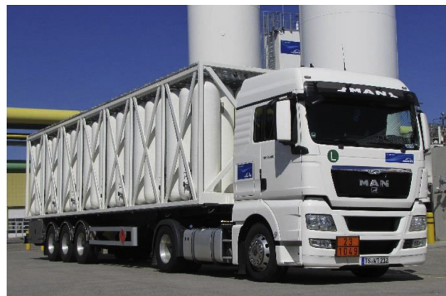
Fig. 1 – State of the art vehicle for the transport of hydrogen in central Europe, based on CPVs (Co. Linde).
