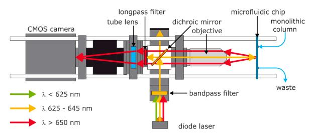
Figure 2. Light paths in the setup with essential optical components.
