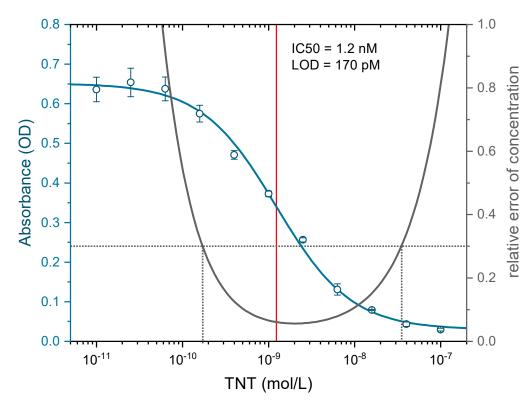
**Figure 5.** Calibration curve (blue) and precision profile (black) of an indirect enzyme-linked immunosorbent assay (ELISA) with the monoclonal antibody A1.1.1. The analyte TNT was determined in quadruplicates.
