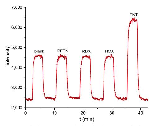
**Figure 8.** Biosensor-based cross-reactivity test for the high explosives pentaerythritol tetranitrate (PETN), 1,3,5-trinitroperhydro-1,3,5-triazine (RDX), octahydro-1,3,5,7-tetranitro-1,3,5,7-tetrazocine (HMX), and TNT at 5 nM. Only 2,4,6-trinitrotoluene (TNT) shows a positive signal.
