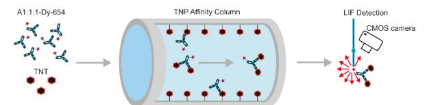
**Figure 1.** A biosensor based on an immunofluorometric assay: The monoclonal antibody A1.1.1 against 2,4,6-trinitrotoluene (TNT) is labeled with the fluorescent dye Dy-654. This conjugate is briefly preincubated with the sample and pumped through the antigen-coated affinity column, which traps free antibody. Only antibody-TNT complexes reach the highly sensitive, laser-induced fluorescence (LIF) detector.
