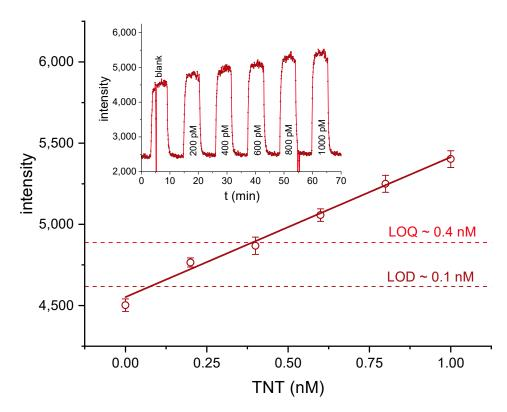
**Figure 7.** Biosensor measurements of TNT solutions in the range from 0 to 1 nM with a linear fit. LOD (3s) and LOQ (10s) were determined as 0.1 nM (20 ppt) and 0.4 nM (90 ppt). Error bars refer to the standard deviation based on subsequent frames. The biosensor signal is shown above.
