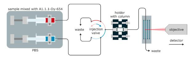
**Figure 3.** Microfluidic setup for the detection of TNT and the cross-reactivity (CR) determination with six-way-valve for continuous flow injection.
