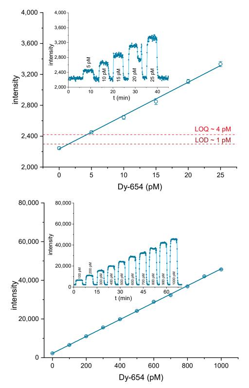
**Figure 6.** Determination of the limit of detection (LOD) (3s) and LOQ (10s) for the fluorescence label Dy-654-COOH (top) and calibration line in the linear range from 4–1000 pM (bottom).
