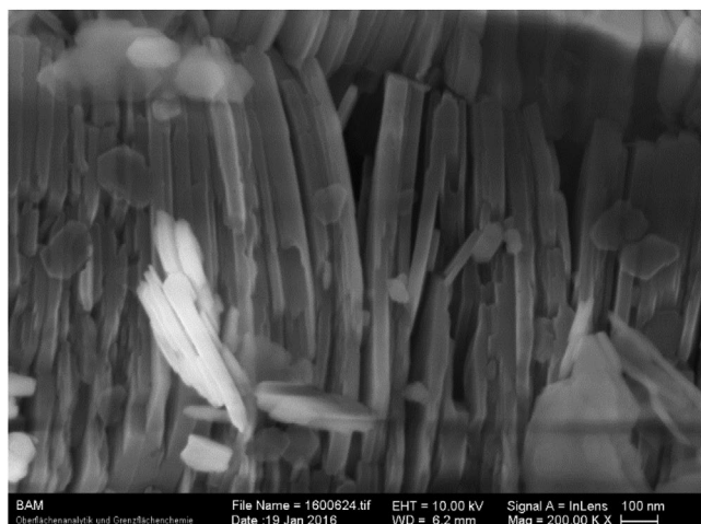
Figure 6. SEM micrograph of Kaolin (IRMM-385).
