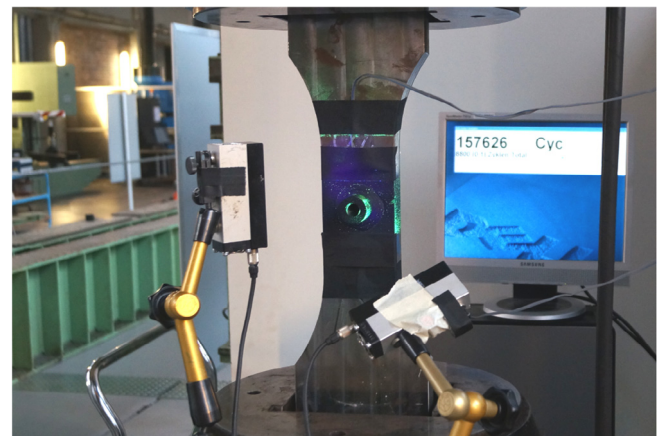
Fig. 5. Test set up for a fillet weld specimen.
