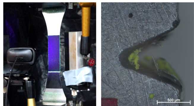
Fig. 2. (a) Tensile test setup; (b) Notch at metal sheet [7].
