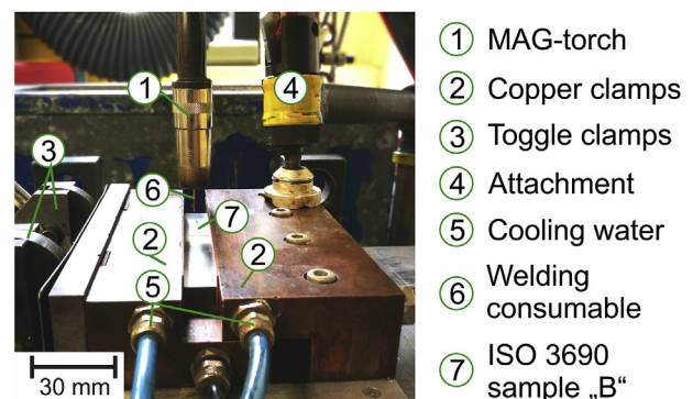
Fig. 4 – Welding fixture for ISO 3690 welding with clamped specimen [55].
