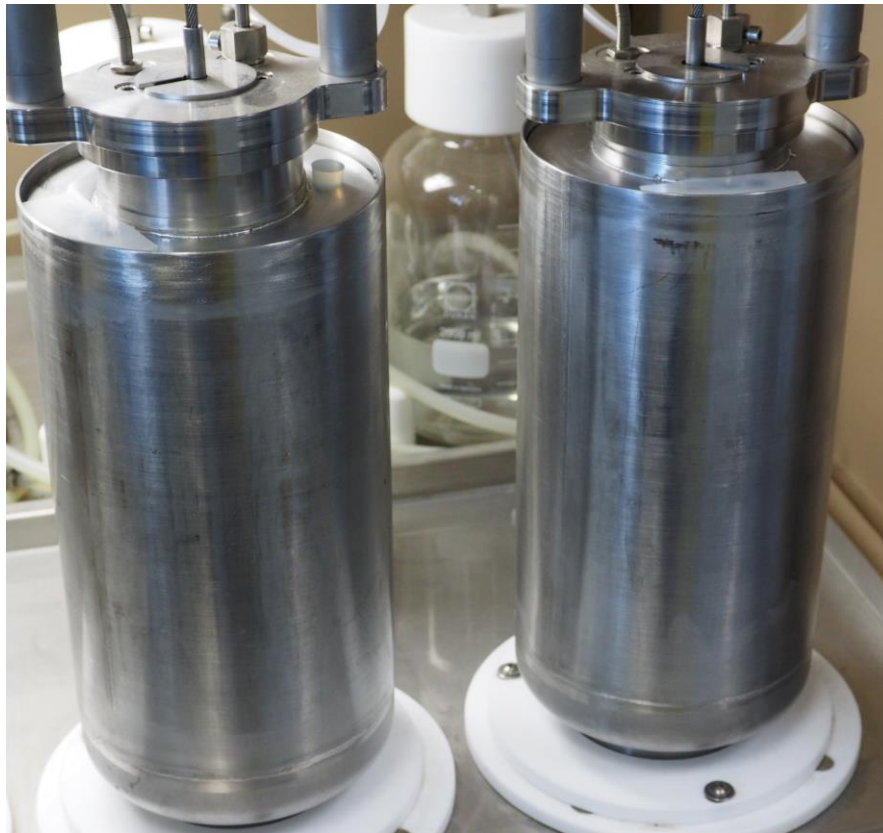
Figure A3.88: Fluid containers for FNCT measurements in air, a) frame container, b) inlay of air container, c) two air containers attached to FNCT device during measurement.
