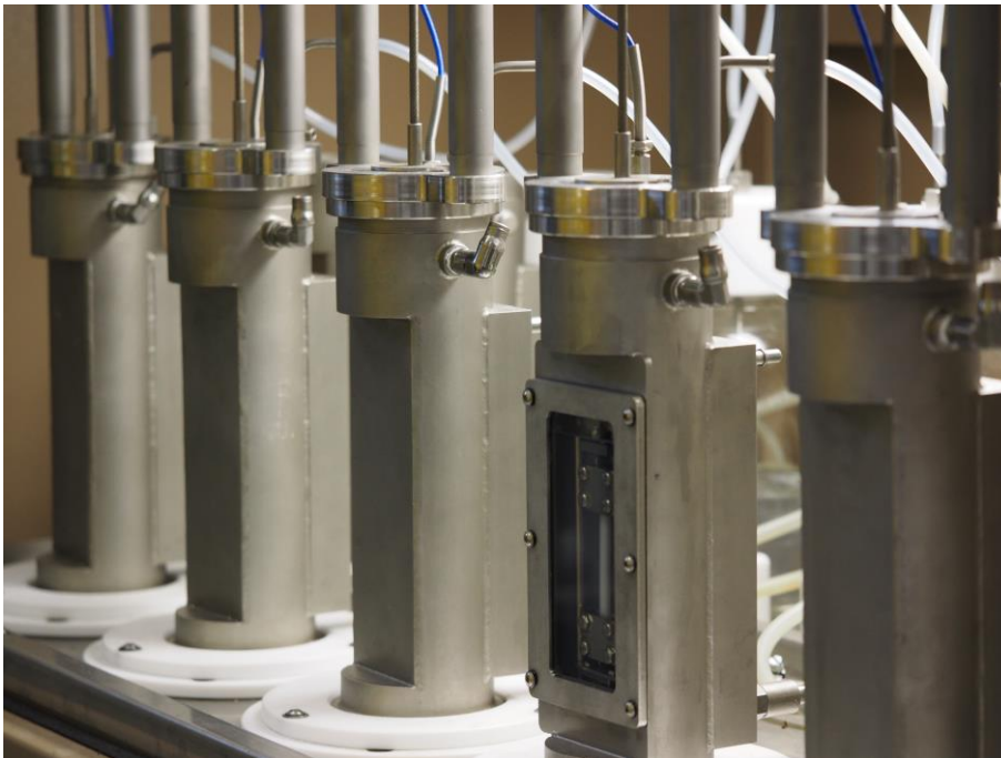
Figure 24: Fluid containers of FNCT device, a) individual container with quartz glass window, b) individual container without window, c) 5 sub-stations, closed fluid containers during measurement.
