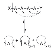
Scheme 45. General principle of backbiting forming cyclics in a reversible reaction.
