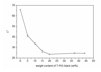
Figure 5.12 CIELAB lightness  $L^*$  of PEU films loaded with different weight contents of T-PIG black. The films were investigated at 23 °C and characterized by a thickness of  $(95 \pm 10) \mu m$ .
