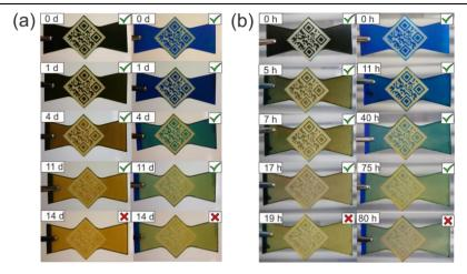
Figure 3.3 Tags after different exposure times to UVA irradiation at 23 °C and 50% air humidity (a) and 60 °C and 16% air humidity (b), respectively. In the ageing series, black tags are shown left and blue tags right. The tags consistently exhibited a vertical color stripe on the left, which was not exposed to UVA light due to clamping. The QR code could be read from all tags with a check mark (top right in the individual images).
