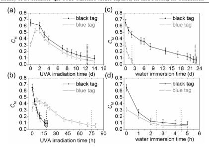
Figure 3.8 Ageing-related changes in Michelson contrast  $C_M$  within the QR code area of black and blue PEU tags. Tags were considered after UVA irradiation at 23 °C and 50% air humidity (a) and at 60 °C and 16% air humidity (b) and water immersion at 23 °C (c) and 60 °C (d). Dotted vertical lines are drawn in for every ageing study to illustrate when QR codes became unreadable (at about a  $C_M$  threshold of 0.1).
