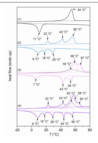
Figure 6.6 DSC thermograms of a solvent cast PEU film (1) and solvent cast PEU films containing 20 wt% of T-PIG blue-43 (2), 20 wt% of T-PIG magenta-65 (3) and T-PIG mixture #4 (4, also see Table 6.1). In every single measurement, the first heating is plotted above the first cooling run. The signals were denoted as "a" (PBA phase changes), "b" (solvent-related phase changes) and "c" (phase changes associated with the color-developer).
