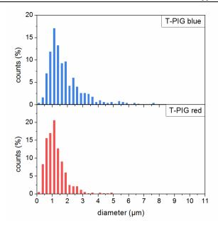
Figure 5.11 Size distribution of as-received powdery T-PIG blue and red as determined from SEM images. The mean particle size was about 1.8 µm for T-PIG blue and 1.2 µm for T-PIG red.
