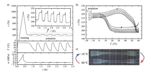
Figure 1.13 Actuation of PEU after training. (a) Evolution of tensile strain  $\varepsilon$ , temperature T and stress  $\sigma$  above time t in five cooling–heating cycles. The inset enlarges the actuation strains. (b) Cyclic evolution of strain versus temperature in five thermal cycles. (c) Trained PEU specimen in the sixth cycle at -10 and 60 °C. Reproduced from Ref. 111 with permission from The Royal Society of Chemistry.
