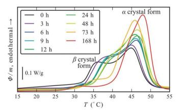
Figure 1.8 DSC thermograms of PEU, showing the first heating run after thermal pretreatment and different times of room temperature annealing, including the assignment of the PBA melting peaks to the  $\beta$  and a crystal form. Reproduced from Ref.<sup>39</sup> with permission from Wiley.
