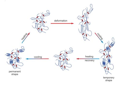
Figure 1.9 Molecular mechanism of programming and recovering a physically cross-linked SMP. Red blocks represent the netpoints formed by hard segments; blue lines represent soft segment.
