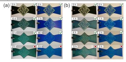
Figure 3.4 Tags after different time intervals of water immersion at 23 °C (a) and 60 °C (b). In the ageing series, black tags are shown left and blue tags right. The QR code could be read from all tags with a check mark (top right in single images).
