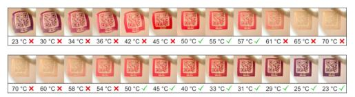
Figure 6.8 Thermo-responsiveness of a type 1 QR code carrier which was surface-colored with T-PIG mixture #4. Starting with the programmed state, the information carrier was heated from 23 to 70 °C (image series above) and cooled to 23 °C (image series below). The symbols on the right side of the temperature values indicate, whether the QR codes were machine-readable or not.
