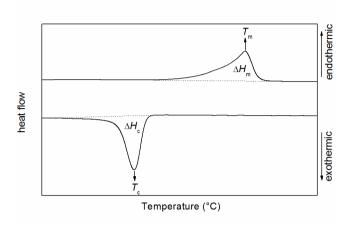
Figure 1.4 Typical DSC thermogram of a polymer with a crystalline phase.
