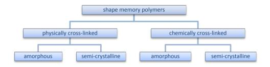
Figure 1.6 Categorization of shape memory polymers.
