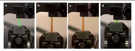
Figure 1.14 Photographs of the one-way shape memory cycle for a 1.5 mg mL<sup>-1</sup> PCO/C18-RG sample (illuminated with 365 nm UV light) during (a) deformation (75 °C, 600 kPa), (b) cooling/fixing (5 °C, 600 kPa), (c) unloading (5 °C, 4 kPa), and (d) recovery (75 °C, 4 kPa). Reproduced from Ref.<sup>151</sup> with permission of The Royal Society of Chemistry.
