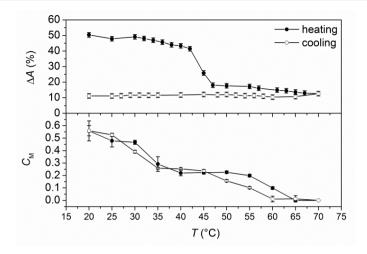
Figure 6.9 Changes in QR code area  $\Delta A$  (top) and Michelson contrast  $C_M$  (bottom), when heating and cooling a programmed type 1 QR code carrier, which was surface-colored with T-PIG mixture #4.
