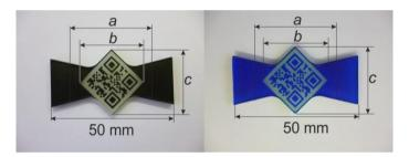
Figure 3.1 Bowtie-shaped PEU tags in black (left) and blue color (right) with identical dimensioning (tag thickness of 2 mm), drawn in a QR code-related longitudinal and transversal length ( $b_0 = c_0 = 25.3 \text{ mm}$ ) and functionalization-related clamping distance  $a_0 = 30 \text{ mm}$ . The QR code contains the information "BAM QRM-Label".
