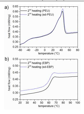
Figure 2.9 DSC thermograms of the 2<sup>nd</sup> heating scan for neat PEU (black line) and surface-dyed PEU (sd-PEU, dotted blue line) (a), and for neat EBP (black line) and surface-dyed EBP (sd-EBP, dotted blue line) (b). The sorption percentages of Victoria Blue B were 0.17 wt% with PEU and 0.18 wt% with EBP, respectively
