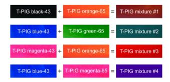
Figure 6.13 Solvent cast PEU films containing 20 wt% of one sort of T-PIG with a CST of 43 °C (left column), 20 wt% of another sort of T-PIG with a CST of 65 °C (column in the middle) and 1:1 mixtures of both (right column). The films had uniform thicknesses of (65  $\pm$  5)  $\mu$ m. The images were recorded at 23 °C.
