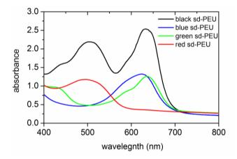
Figure 3.11 Visible absorption spectra of purely black (composed of a Victoria Blue B, Basic Green 1 and Basic Red 28 mixture), blue (Victoria Blue B), green (Basic Green 1) and red (Basic Red 28) surface-dyed PEU.
