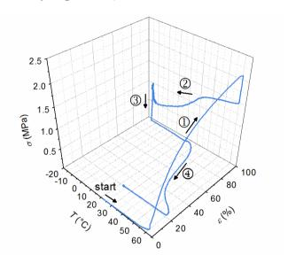
**Figure 1.11** Cyclic thermo-mechanical measurement of a PEU, showing one cycle including elongation ①, strain fixing ②, unloading ③ and strain recovering ④.
