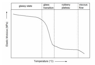
Figure 1.3 Typical DMA measurement of an amorphous polymer.
