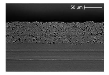
Figure 6.15 Scanning electron micrograph of a PEU surface layer containing T-PIG mixture #4 atop PEU substrate.
