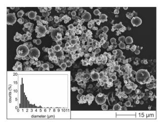
Figure 5.3 SEM image of as-received powdery T-PIG black; the inset gives the size distribution of the microcapsules.
