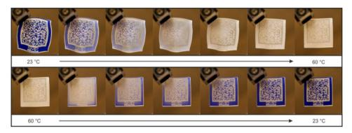
Figure 5.9 Thermo-responsiveness of a multifunctional QR code carrier. Starting with the programmed state, the information carrier was heated from 23 to 60 °C and cooled to 23 °C, at which the QR code became machine-readable. Uniform heating and cooling rates of  $\pm 4$  °C min<sup>-1</sup> were selected.
