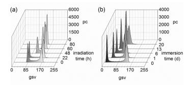
Figure 3.7 Grayscale histograms: ageing-dependent changes in grayscale value (gsv) and pixel counts (pc) of a blue tag, UVA irradiated at 60 °C and 16% air humidity (a), and a black tag, hydrolytically aged at 23 °C (b).
