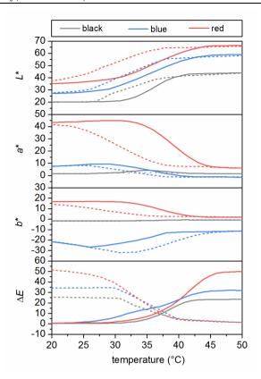
Figure 5.13 Temperature-dependence of the colorimetric properties of PEU films, containing either 20 wt% of T-PIG black, blue or red. The thickness of the films was  $(95 \pm 10) \mu m$ . The temperature evolution in lightness  $L^*$ , the opponent color values  $a^*$  and  $b^*$  and the color difference  $\Delta E$  is given during heating (continuous lines) and cooling (dashed lines).
