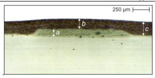
Figure 6.18 Microscopic image of a type 2 QR code carrier containing T-PIG green-65 in a laser-engraved bottom layer and T-PIG black-43 in a continuous cover layer. Layer thicknesses of  $a = (119 \pm 6) \ \mu m$ ,  $b = (152 \pm 6) \ \mu m$  and  $c = (211 \pm 6) \ \mu m$  were determined.
