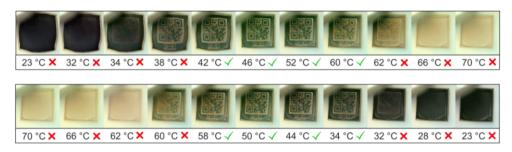
Figure 6.11 Thermo-responsiveness of a type 2 QR code carrier containing T-PIG green-65 in a laser-engraved bottom layer and T-PIG black-43 in a cover layer. Starting with the programmed state, the information carrier was heated from 23 to 70 °C (image series above) and cooled to 23 °C (image series below). The symbols on the right side of the temperature values indicate, whether the QR codes were machine-readable or not.
