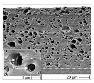
**Figure 5.6** SEM image showing the cryomicrotome section profile of a PEU cover layer filled with T-PIG black (~ upper 100 μm cutout, above the dotted line) atop PEU plaque (~ lower 10 μm cutout, below the dotted line). The inset shows highly resolved cavities.
