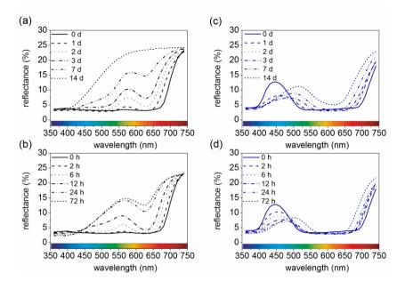
Figure 3.6 Reflectance as a function of wavelength  $\lambda$  for black ((a) and (b)) and blue ((c) and (d)) surface-colored PEU samples after different UVA ageing periods at 23 °C ((a) and (c)) and 60 °C ((b) and (d)), respectively.
