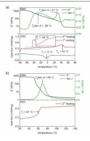
Figure 2.3 Thermal and mechanical properties of neat PEU (a) and EBP (b) as determined by DMA and DSC. For both polymers, the temperature-dependence of E' (black curve) and  $\tan \delta$  (green curve) is plotted above. The DSC thermograms are given below; they include the 1<sup>st</sup> cooling scan (blue curve) and 2<sup>nd</sup> heating scan (red curve with enlarged glass transition region provided by the inset) for PEU and the 2<sup>nd</sup> heating scan for EBP.
