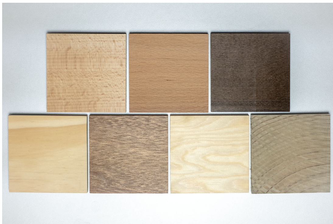
FIGURE 1 Specimen tested—top row: Beech, Belmadur beech, and Thermo beech; bottom: Pinus radiata , Meranti, Pinus sylvestris L., and Accoya [Colour figure can be viewed at wileyonlinelibrary.com ]
