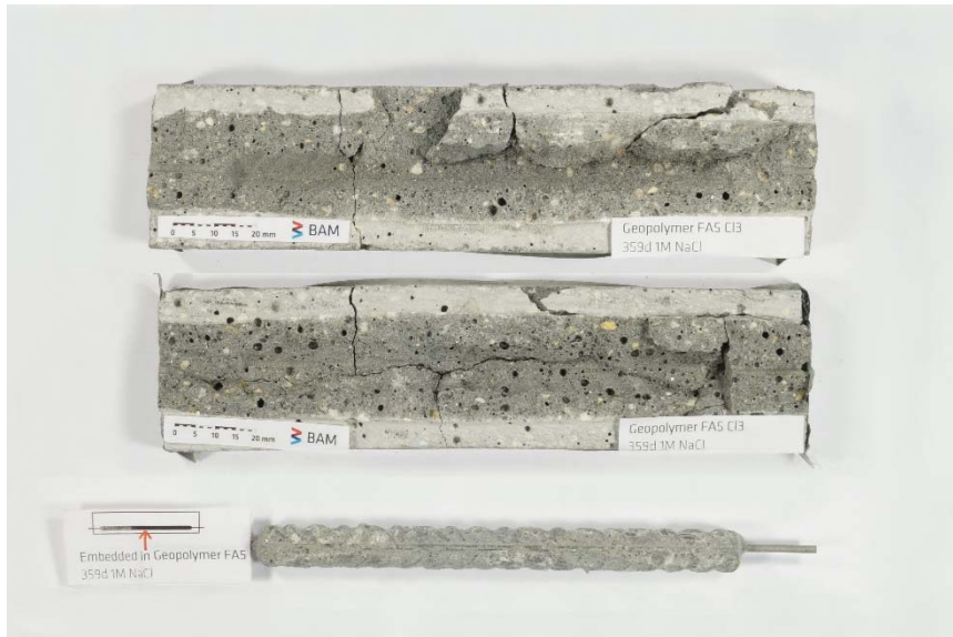
Figure S7. Mortar specimen FA-Cl 3 and embedded steel rebar split after depassivation of the steel was detected.
