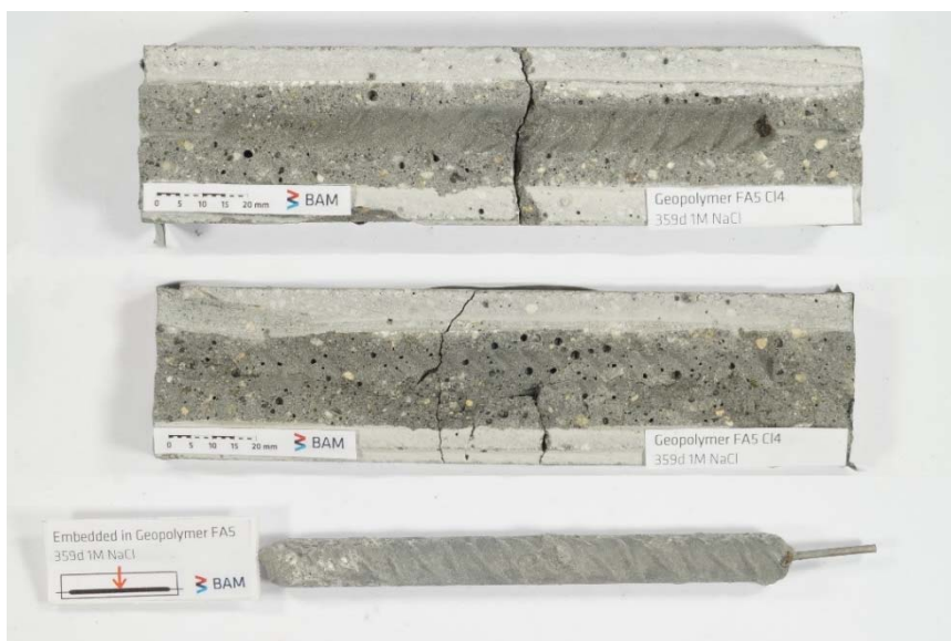
Figure S8. Mortar specimen FA-Cl 4 and embedded steel rebar split after depassivation of the steel was detected.
