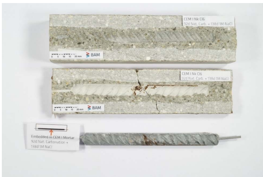
Figure S28. Mortar specimen CEM-A-CI 6 and embedded steel rebar split after depassivation of the steel was detected.
