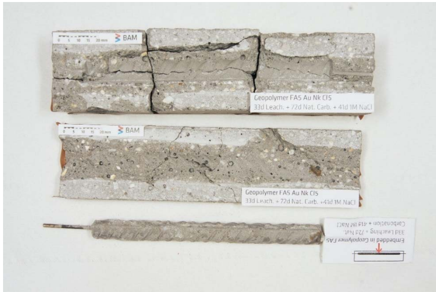
Figure S21. Mortar specimen FA-L-A-Cl 5 and embedded steel rebar split after depassivation of the steel was detected.
