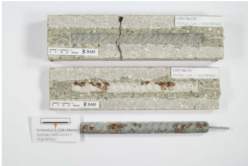
Figure S25. Mortar specimen CEM-Cl 3 and embedded steel rebar split after depassivation of the steel was detected.
