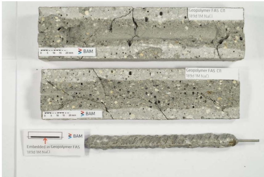
Figure S5. Mortar specimen FA-Cl 1 and embedded steel rebar split after depassivation of the steel was detected.
