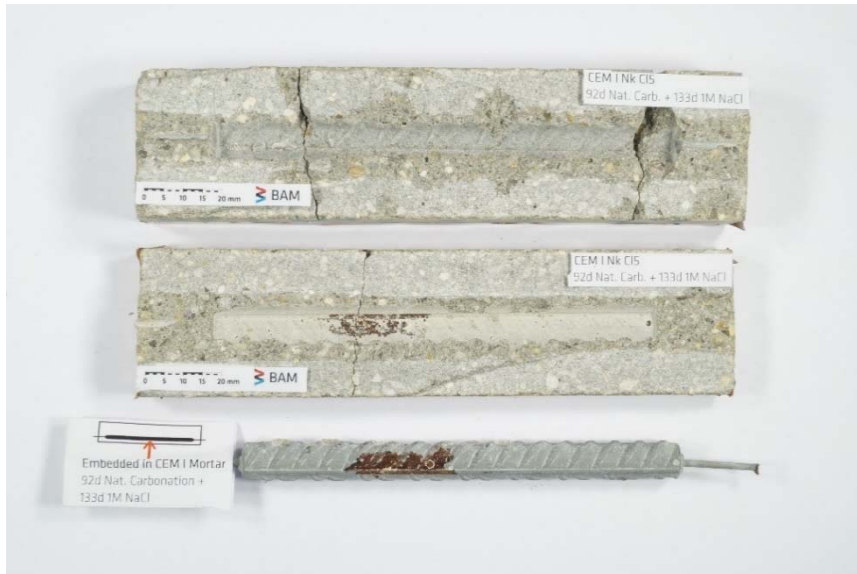
Figure S27. Mortar specimen CEM-CI 5 and embedded steel rebar split after depassivation of the steel was detected.
