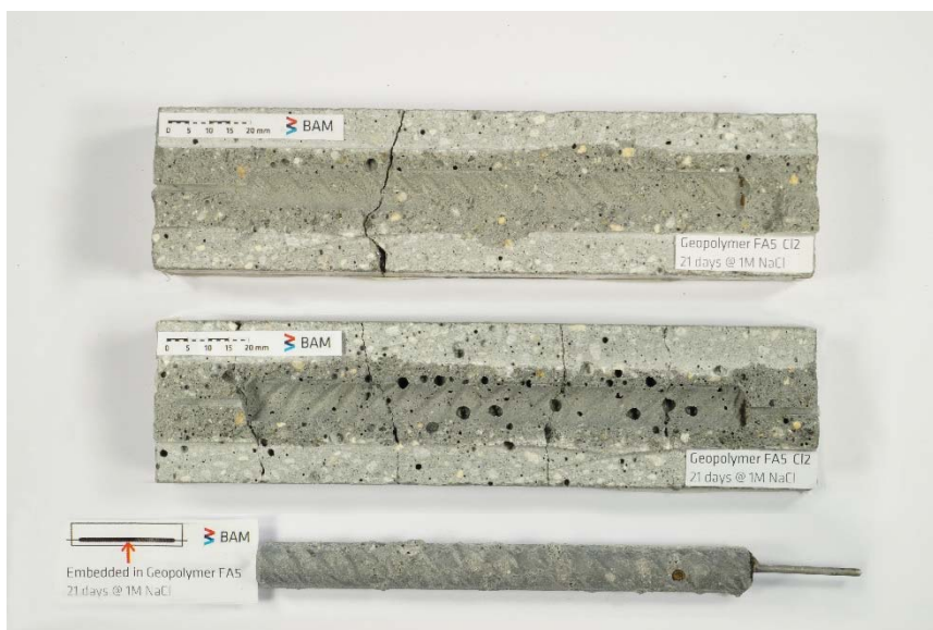
Figure S6. Mortar specimen FA-Cl 2 and embedded steel rebar split after depassivation of the steel was detected.
