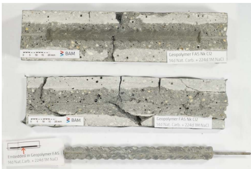
Figure S10. Mortar specimen FA-Cl 8 and embedded steel rebar split after depassivation of the steel was detected.
