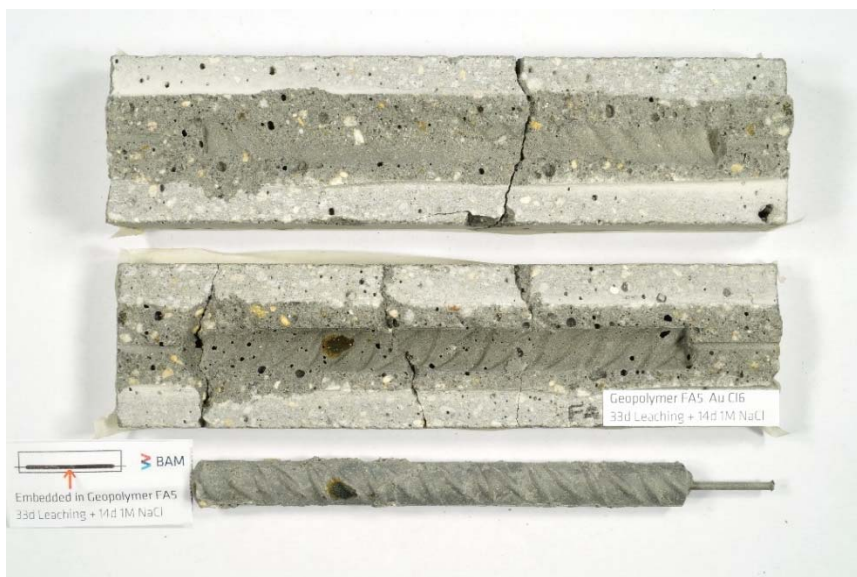
Figure S16. Mortar specimen FA-L-Cl 6 and embedded steel rebar split after depassivation of the steel was detected.
