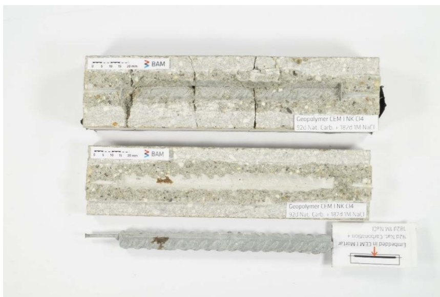
Figure S26. Mortar specimen CEM-Cl 4 and embedded steel rebar split after depassivation of the steel was detected.
