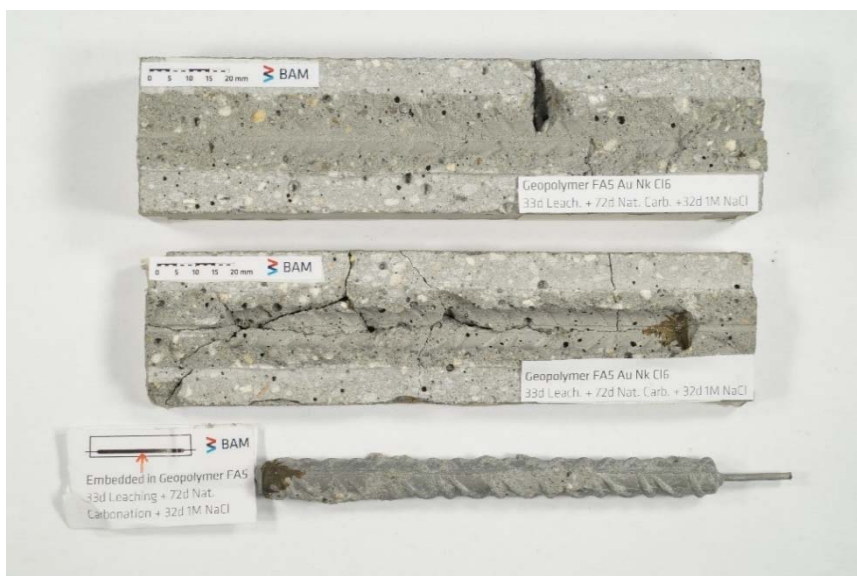
Figure S22. Mortar specimen FA-L-A-Cl 6 and embedded steel rebar split after depassivation of the steel was detected.
