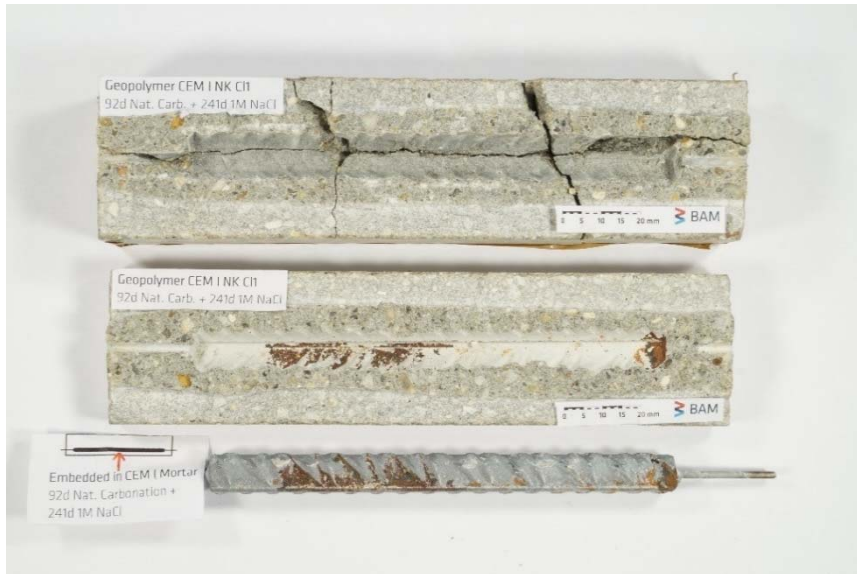
Figure S23. Mortar specimen CEM-CI 1 and embedded steel rebar split after depassivation of the steel was detected.
