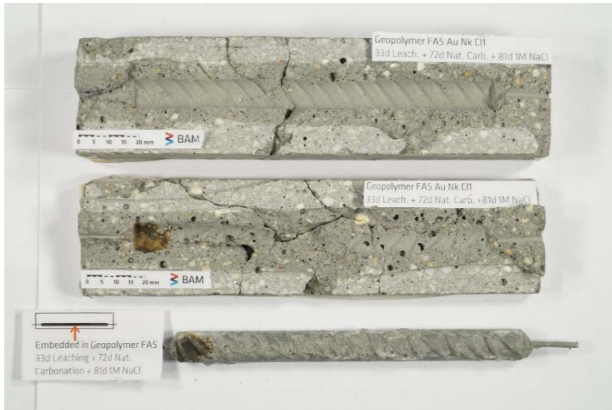
Figure S17. Mortar specimen FA-L-A-Cl 1 and embedded steel rebar split after depassivation of the steel was detected.
