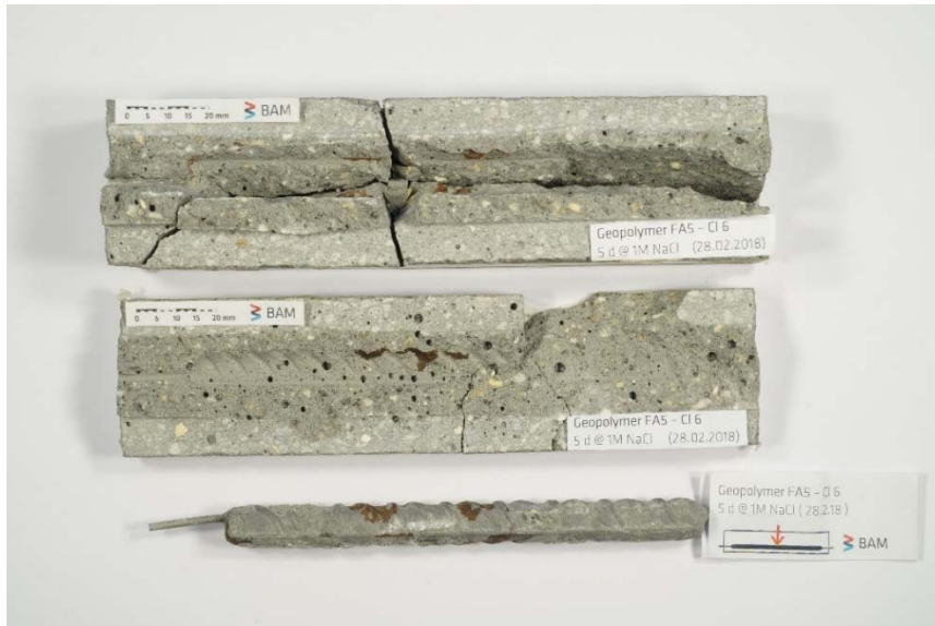
Figure S9. Mortar specimen FA-Cl 6 and embedded steel rebar split after depassivation of the steel was detected.
