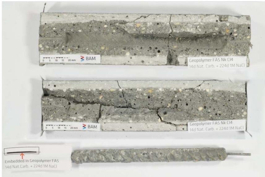
Figure S11. Mortar specimen FA-Cl 10 and embedded steel rebar split after depassivation of the steel was detected.
