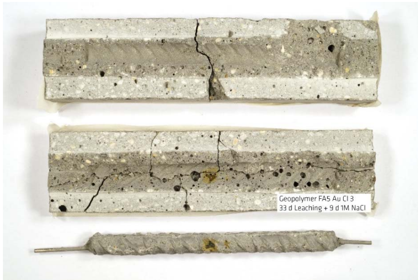
Figure S13. Mortar specimen FA-L-CI 3 and embedded steel rebar split after depassivation of the steel was detected.
