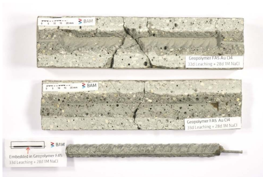
Figure S14. Mortar specimen FA-L-CI 4 and embedded steel rebar split after depassivation of the steel was detected.
