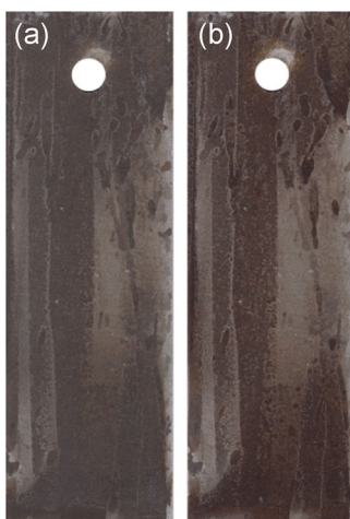
FIGURE 8 Appearance of the surfaces of AlSi1.2Mg0.4 mechanically ground with Abrasive C: (a) after 48-hr condensed water test, (b) after 48-hr condensed water test and subsequent pickling with nitric acid for 10 min [Color figure can be viewed at wileyonlinelibrary.com ]
