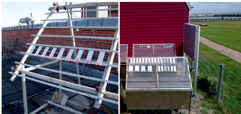
FIGURE 2 Exposed AlSi1.2Mg0.4 sheets on the roof of the BAM main building in the city of Berlin (left, urban atmosphere) and on the island of Heligoland (right, marine atmosphere) [Color figure can be viewed at wileyonlinelibrary.com ]
