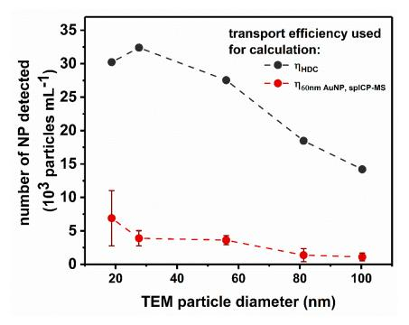
**Figure 2.** Au-NP number concentrations for different sizes as obtained by HDC-spICP-MS considering the size-dependent transport efficiency: (1) according to the TS (red dots,  $\eta_{60nm AuNP}$ ), (2) size-dependent (black dots,  $\eta_{HD}$ ).
