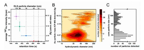
**Figure 3.** (**A**) Cross calibration of the HDC-spICP-MS with hydrodynamic (DLS) and the particle mass per event based on the core diameters from TEM. (**B**) Spike fractogram of a mixture of 4 differently sized Au-NPs. (**C**) Frequency based distribution of measured core particle sizes.
