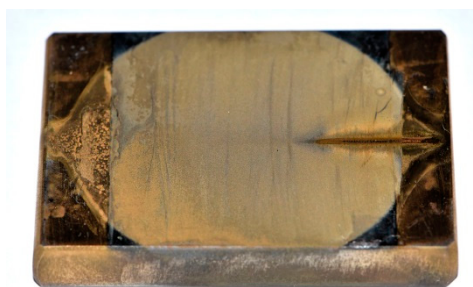
Figure 6. Photograph of a specimen after an in-situ energy-dispersive X-ray diffraction (EDXRD) experiment in an Oxyfuel atmosphere at 278 K and 1 bar for 15 h. The circular spot on the surface of the specimen reveals the reaction zone generated during the corrosion experiment. On the left and right margins of the specimen, the thin Au layer are still visible. The beam was entering from the left side, touching in the center and then leaving off the right side, generating a distinctly altered zone.
