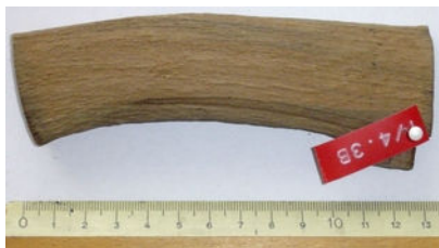
Fig. 1. Wooden specimen from a sunken ship wreck. Curved shape deformation as a result of dehydration.
