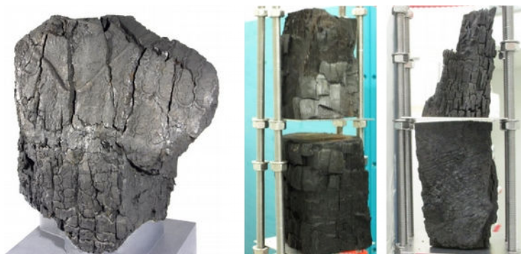
Fig. 3. Heat damaged torso that was not transportable and mock-ups for testing conservation protocols. The treated specimens (bottom) and the untreated controls (top) were imaged together. The treatment consisted out of soaking with boiled linseed oil (centre) or polyvinyl butyral (PVB, right).
