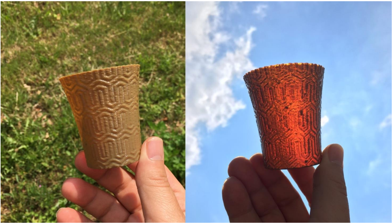
Figure S4. The 3D printed AgNP@PVA dichroic material under sunlight, reflected light on the left and transmitted light on the right.
