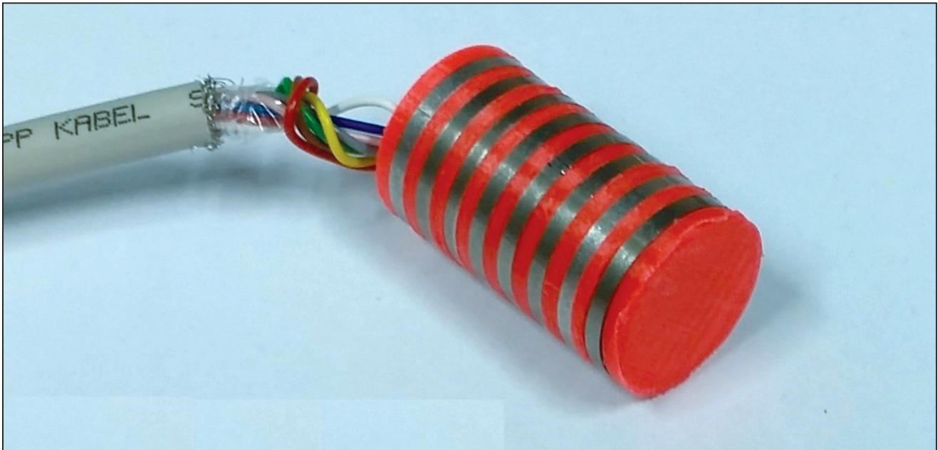
Fig. 2: Embedded multi-ring-electrode before concreting
