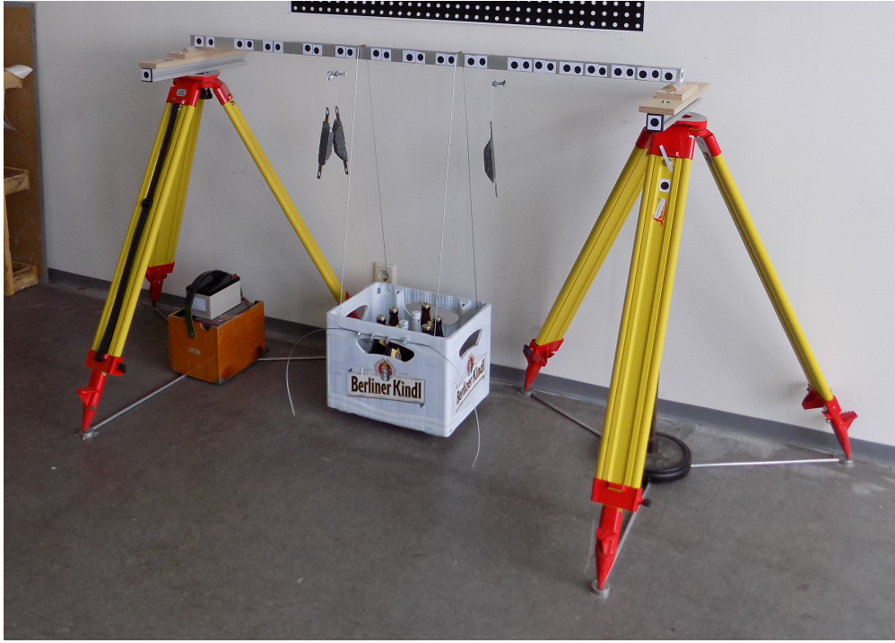
Figure 5.12: A six-point bending test apparatus for an aluminium beam specimen. This test device was partly enhanced by scrap such as lead battery, dumbbell, plastic box.
