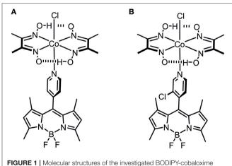
FIGURE 1 | Molecular structures of the investigated BODIPY-cobaloxime complexes 1 (A) and 2 (B).
