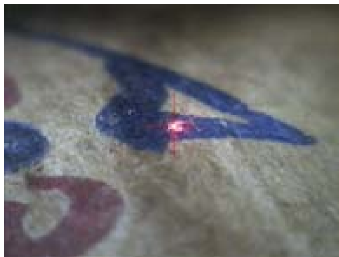
Fig. 5 XRF analysis of the blue ink of M 233.
