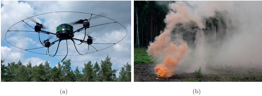
Figure 3.1: (a) Airrobot AR100-B micro-drone in flight. (b) Visualized disturbance induced by the rotors of the Airrobot AR100-B micro-drone using an AX-430 orange colored smoke bomb (photo taken at BAM TTS).
