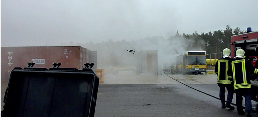
Figure 9.1: Micro-drone monitoring relevant parameters (gas concentrations, wind, temperature, and humidity), while the fire brigade extinguishes a bus on fire. Photo taken at BAM TTS during an artificial fire scenario.
