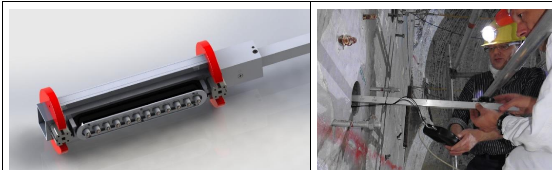
Figure 4. Ultrasonic borehole probe and deployment in a former salt mine (Niederleithinger, 2019).
