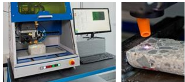
Fig. 1. Overall view of the LIBS laboratory system (left). Detailed view on the sample surface with plasma and nozzle of helium feeder (right).
