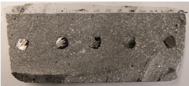
Fig. 2. Galvanic anode/mortar probe cut broadside for LIBS measurements
