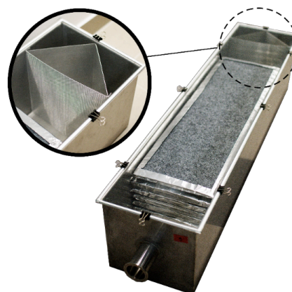
Fig. 4. CLIMPAQ - Emission chamber with carpet samples (B)
