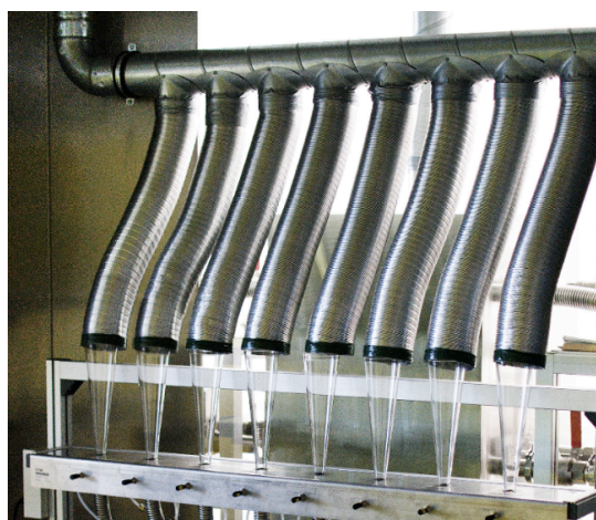
Fig. 5. Reference scale of the HTW-Berlin with individual connecting piece for exhaust air for each funnel.
