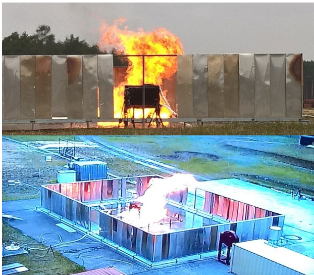
Fig. 6 GFRP tank under fully developed fire
