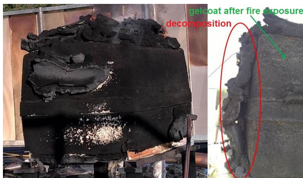
Fig. 7 Heat-related decomposition of the fire protective thermoplastic foil applied on the outer tank surface
