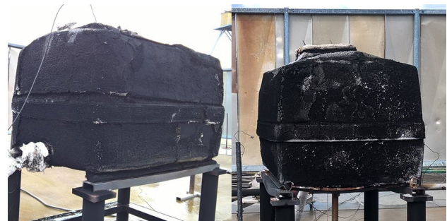
Fig. 8 Inspection after fire tests—GFRP tanks with a protective coating of type A (left) and type B (right)
