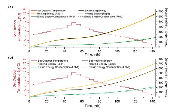
**Figure 6.** Cumulated heating energy and cummulated electric energy consumption of: (**a**) HP#2 measured two times in the same laboratory; and (**b**) HP#1 measured in different laboratories, Lab 1 and Lab 2, respectively.
