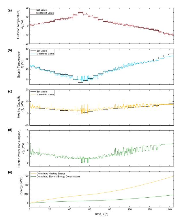
**Figure 3.** Results of the dynamic test for HP#1 (GSHP) using the climate box: (**a**) outdoor temperature  $\vartheta_o$ ; (**b**) supply temperature  $\vartheta_s$ ; (**c**) heating capacity  $\dot{Q}_h$ ; (**d**) electrical power consumption  $P_{el}$ ; and (**e**) cumulated energies (thermal  $Q_h$  and electrical  $E_{el}$ ).
