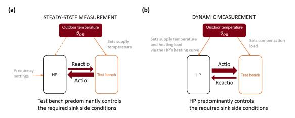
Figure 1. Methodology of: (a) the steady-state test according to EN 14825; and (b) the dynamic test.
