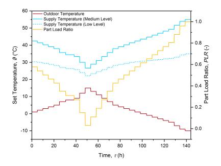
**Figure 2.** Profiles of the outdoor temperature (red line), supply temperature at medium (blue solid line) and low level (blue dashed line) and the corresponding part load ratio (yellow line).
