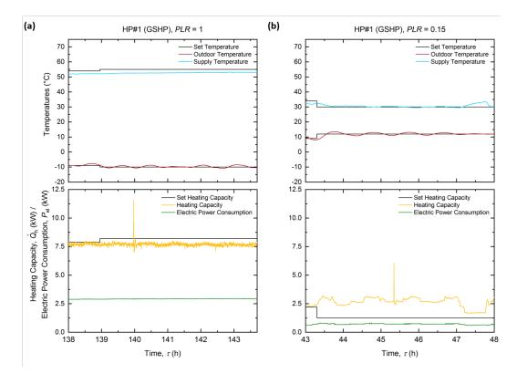
**Figure 4.** Measurement of a GSHP using the climate box at: (**a**) rated capacity (PLR = 1); and (**b**) part load (PLR = 0.15).
