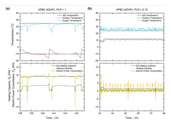
**Figure 5.** Measurement of an ASHP using the climate box at: (**a**) rated capacity (PLR = 1); and (**b**) part load (PLR = 0.15).
