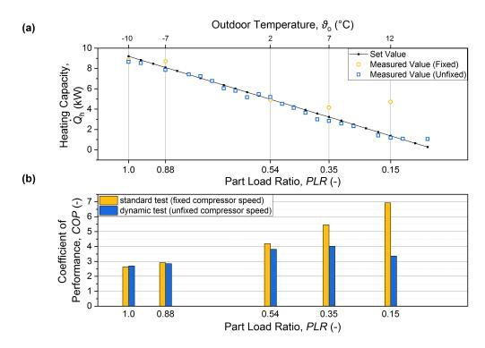
**Figure 8.** (a) Average heating capacity; and (b) Coefficient of Performance results of HP#2 for different PLRs determined with the dynamic method (unfixed compressor speed: VFD or ON/OFF operation) and according to EN 14825 (fixed compressor speed).
