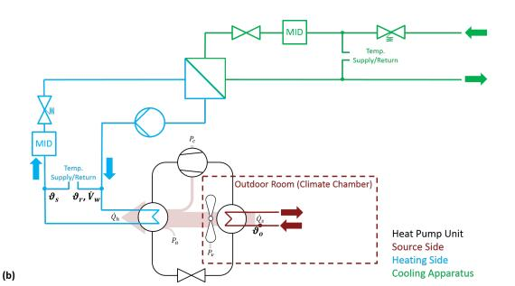
Figure A1. Experimental Setup for: (a) GSHP; and (b) ASHP applications.
