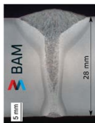
Fig. 6. 28 mm thick single-pass welded sample with electromagnetic weld pool support system
