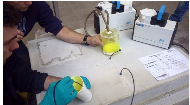
Fig. 10. Filling the air voids with fluorescent resin using a vacuum pump
