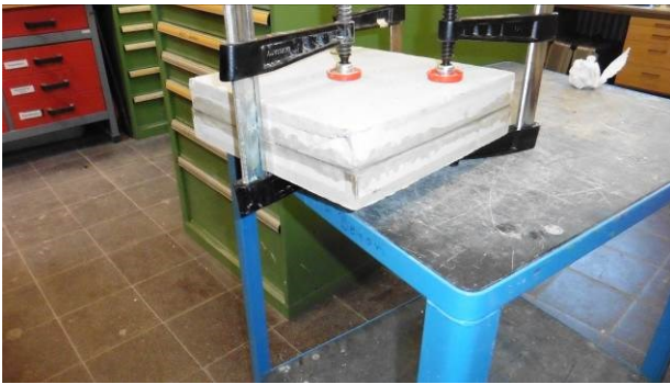
Fig. 9. Two fixed concrete plates with a small air gap between each other to simulate a delamination
