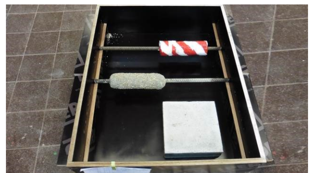
Fig. 8. Prepared test specimen with different artificial defects before pouring concrete
