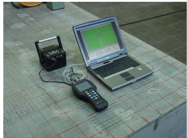
Fig. 4. Standard Ultrasonic equipment for concrete inspection consisting of three basic components (handheld, probe, computer for data analysis)
