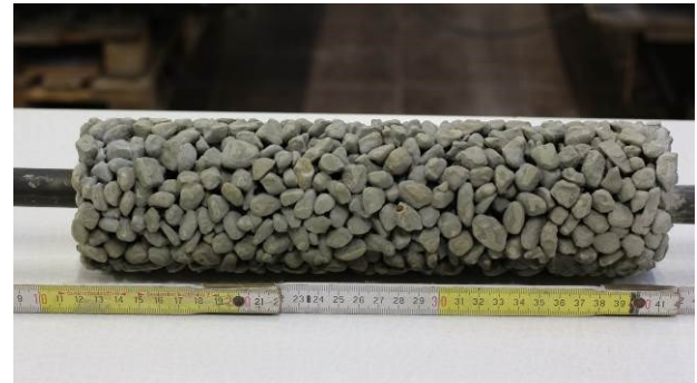
Fig. 7. Artificial honeycomb on reinforcement bar without finished coating during production process
