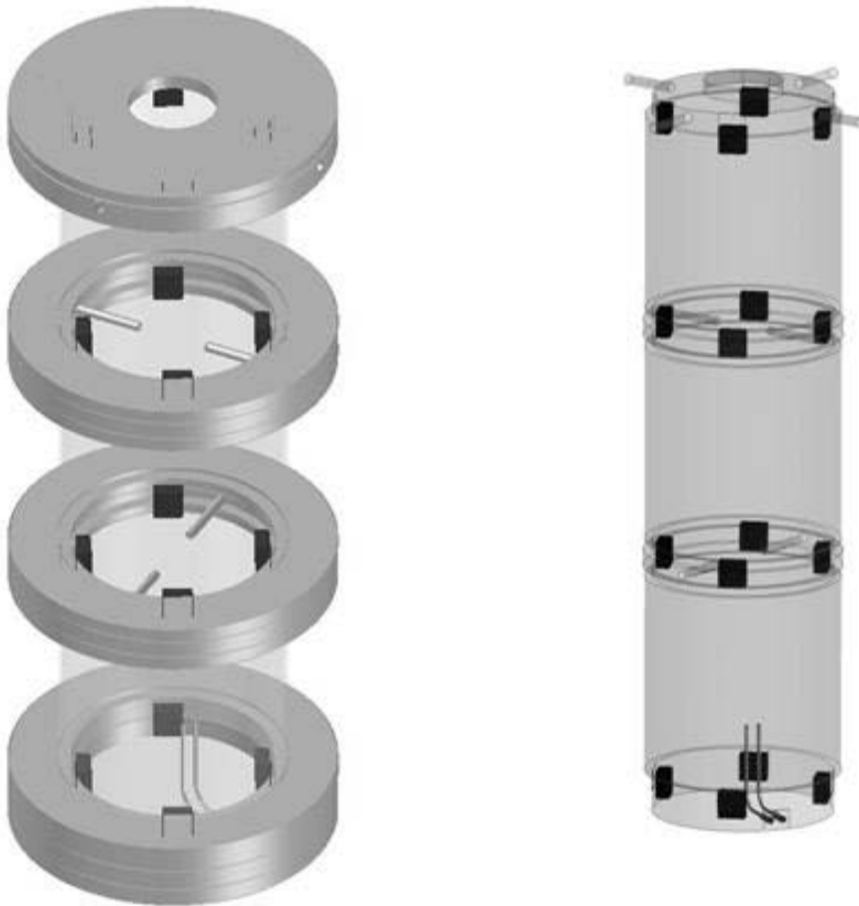
Figure 7-7. CAD model (left) and CFD model (right).
