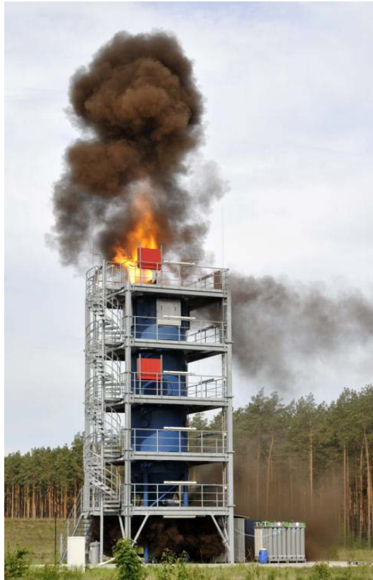
Figure 2-2. Vented dust explosion in a silo (photo: BAM).
