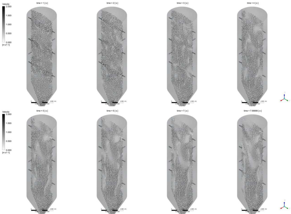
Figure 7-22. Velocity from second 1 to second 8, homogenous injection.
