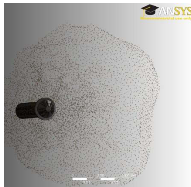
Figure 7-21. Injected dust as point cloud.
