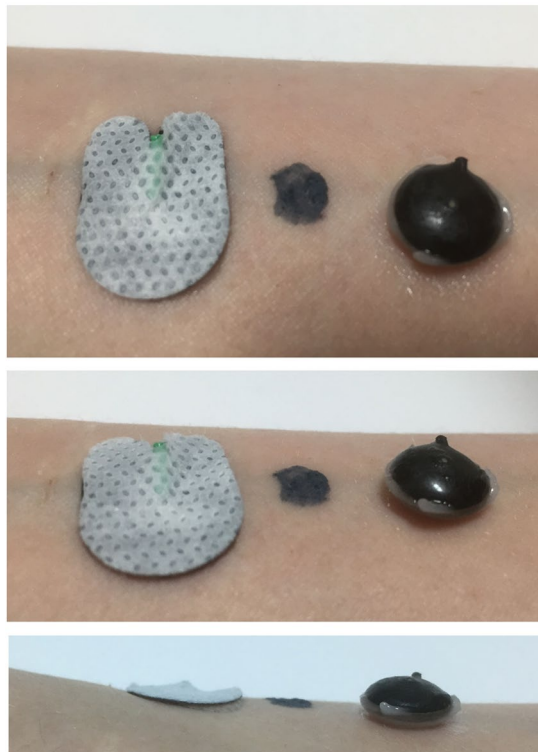
Figure 1. Three types of EEG electrodes on human skin. On the left, a relatively flat hydrogel electrode, the PEDOT polymer electrode (4 mm diameter) in the middle and on the right side a Ag/AgCl cup electrode with conductive gel (photograph created by Jürgen Bergeler).
