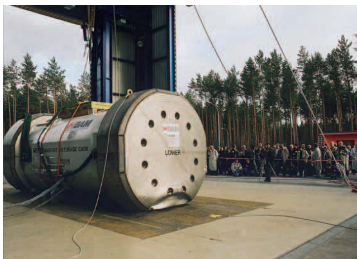
5 Spent fuel transport container after a drop test from a height of 9 metres on an unyielding base
