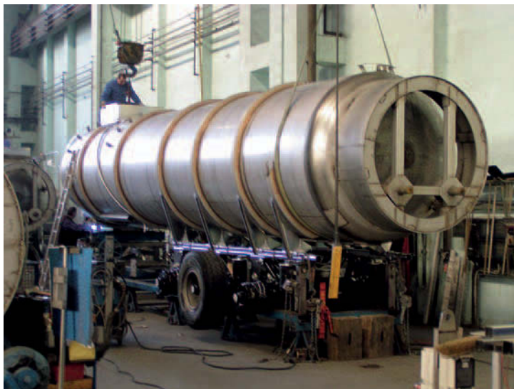
22 Tanker made of special high-grade steel
