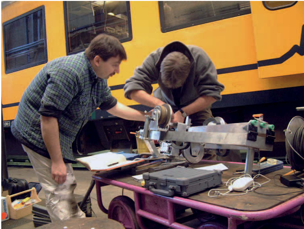
25 Testing the eddy current technology on a rail test train
