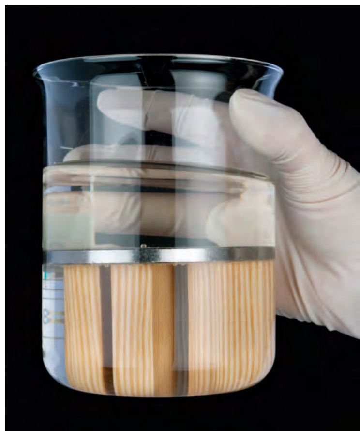
Test assembly for the investigation of leaching processes
