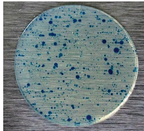
Result of the KorroPad test after 15 minutes
