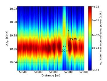
Figure 7. Color plot of logarithmized normalized reflected power of a 100 m fiber section at 51.7 km in a temperature chamber at 60 °C.
