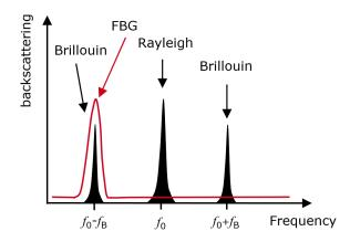
**Figure 2.** Black: Schematic of the frequency spectrum components without filtering, red curve: Filtering by the FBG of Rayleigh scattering and the upper sideband generated by the MZM1 of the probe.
