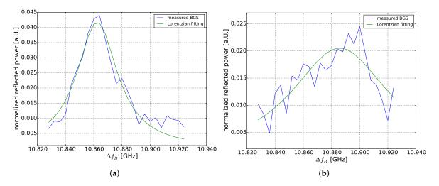
Figure 5. (a) BGS at 50 km at room temperature (b) BGS at 51.7 km within the heated section.
