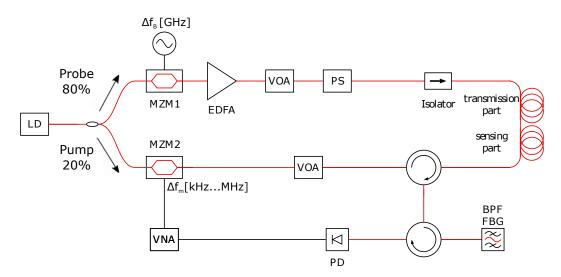
**Figure 1.** BOFDA sensor setup. LD: laser diode; MZM: Mach–Zehnder modulator; EDFA: erbium-doped fiber amplifier; VOA: variable optical attenuator; PS: polarization scrambler; SMF: single mode fiber (for detailed configuration, see Figure 3); BPF FBG: bandpass filter fiber Bragg grating; PD: photodiode; VNA: vector network analyzer.
