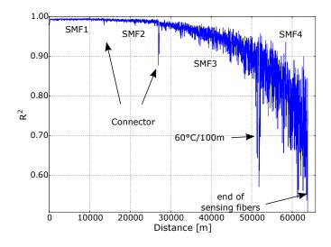
**Figure 6.**  $R^2$  of fitting with Lorentzian function over distance.
