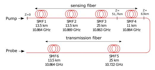
**Figure 3.** Structure of the fiber loop. Information about length and  $\Delta f_B$ .
