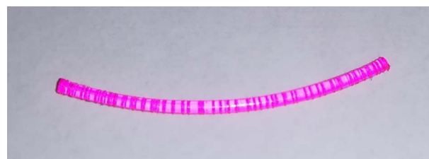
Fig. 6. Lateral photo of the over-annealed 3 cm long ESKA GK-40 sample that was soaked in the doping solution for 93 h at 20 °C.
