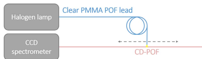
Fig. 9. Schematic illustration of the experimental setup used for the CD-POF side-illumination fluorescence measurement.
