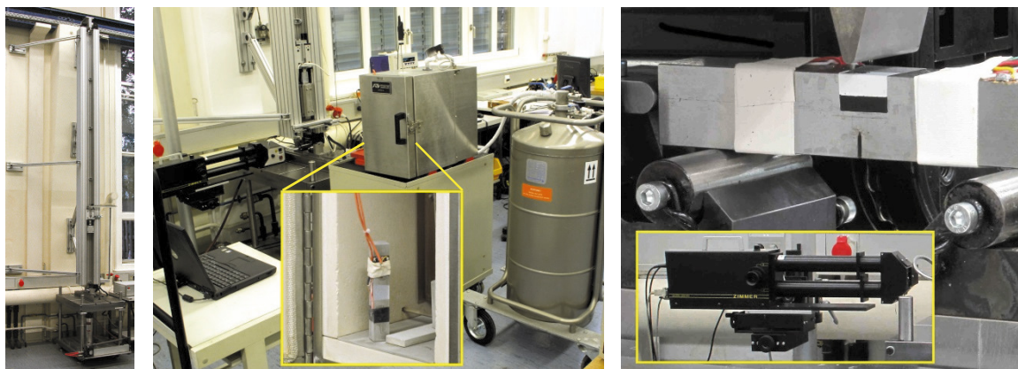
Fig. 1. BAM drop tower test facility (left: total view, middle: tempering chamber for cooling with liquid nitrogen, detail with specimen inside, right: triple point bending loading fixture with instrumented specimen and electro-optical camera for displacement measurement).
