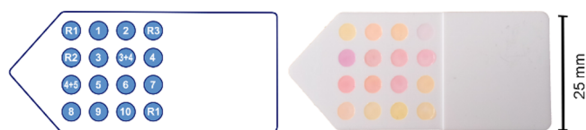
Figure 2. Final configuration of the sensor and reference spots containing 1–10 and R1–R3 on the PMMA strip. The 16 wells were arranged in a 4 \times 4 fashion, with a grid size of 8 mm. The dimensions of the wells were height = 50 \mu\text{m} , diameter = 5 mm.
