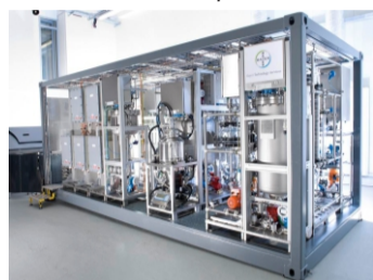
Fig. 1: Containerized modular plant (source: INVITE GmbH)
