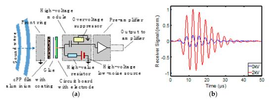
**Figure 2.** (a) Receiver with a high-voltage module that adds an external bias-voltage  $V_{dc}$  to the existing internal voltage  $V_0$  of the ferroelectret film. (b) Receiver signals with a bias-voltage  $V_{dc}$  of 0 V (blue) and 2000 V (red).
