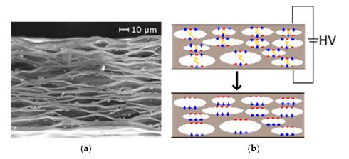
**Figure 1.** (a) Cellular polypropylene (cPP) films have an internal structure with voids which provides low acoustic impedance close to that of air. (©EMFIT Ltd.) (b) The film is polarized with corona discharges. The charge is trapped at the surfaces of the voids creating quasi-permanent polarization equivalent to a voltage  $V_0$ .
