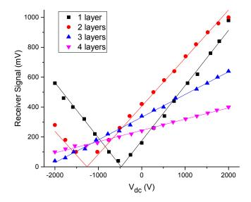
Figure 3. Peak-to-peak signals received with a high-voltage module versus bias-voltage Vdc.
