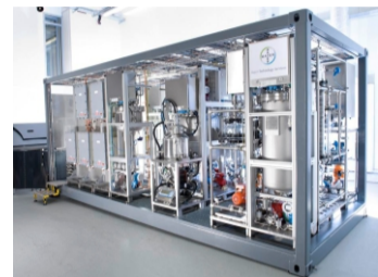
Fig. 1: Containerized modular plant (source: INVITE GmbH)
