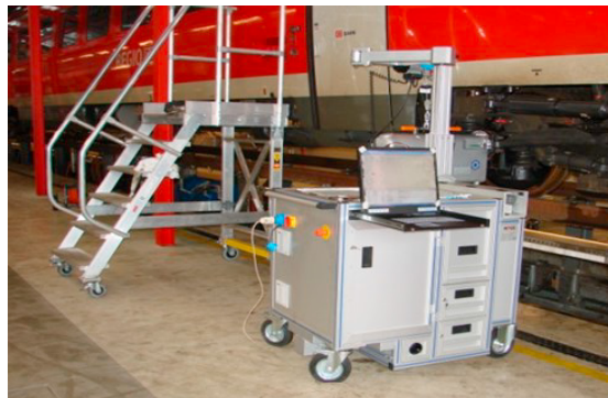
Fig. 1. Example for a mechanized ultrasonic inspection system for the inspection of hollow axles used by Deutsche Bahn
