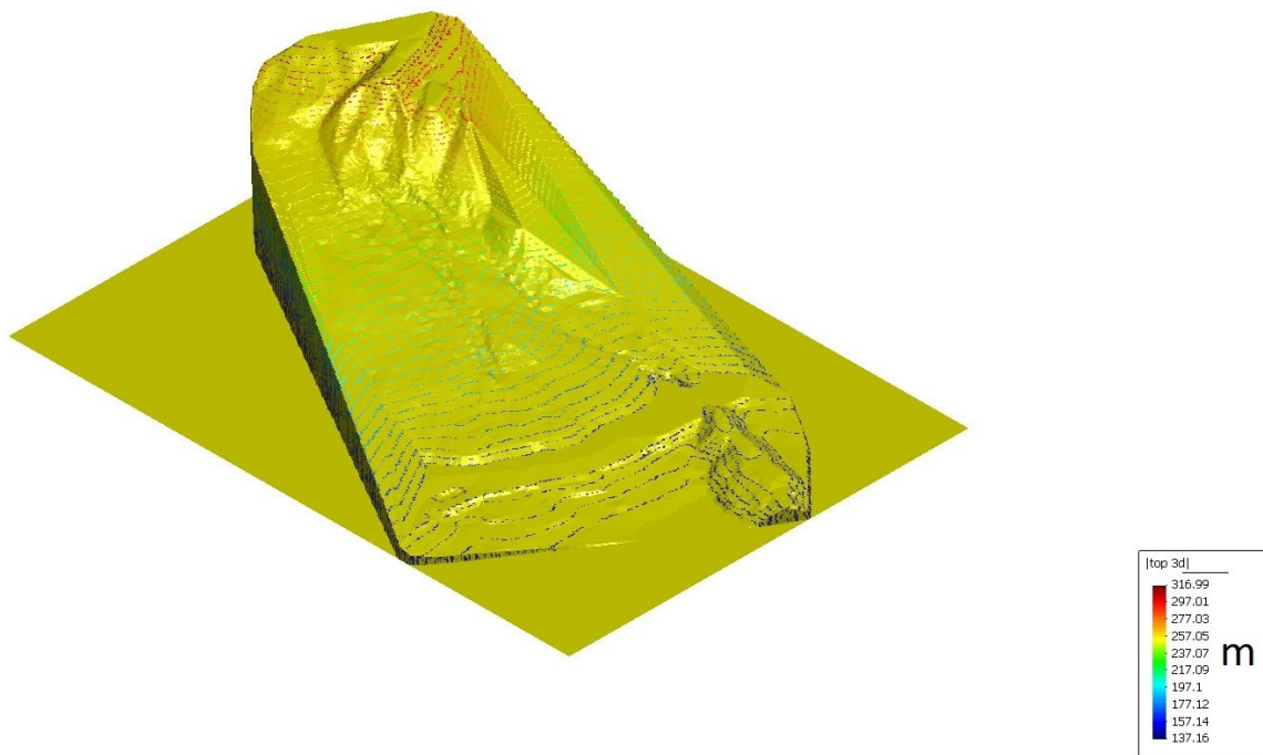
Figure 7. The Aberfan 3D topographic mesh generated using the map of Figure 6 as a starting point. Different colors represent different isolines' height.
