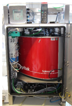
Fig. 1: Concept for process control within a continuous chemical production plant based on an Online-NMR Analyzer
