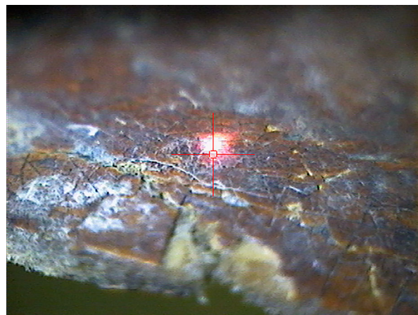
Figure 9 Photomicrograph with laser spot from orpiment as layer on paper, SyrHT 101.
