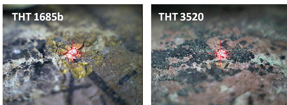
Figure 10 Photomicrographs with laser spot from different Tocharian manuscript fragments, showing different gold applications. Tocharian THT 1685b: gold leaf on white cerussite; Tocharian THT 3520: goldflake (containing Cu and Hg).
