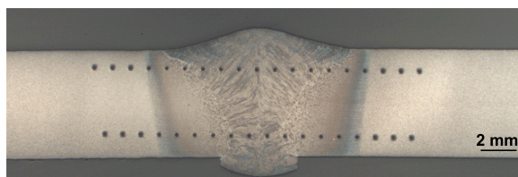
Fig. 4.6: Hardness measurement on a cross-section sample
