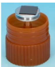
Fig. 1: Universal EDS-CRM prepared using a Si wafer based chip technology.
