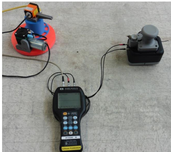
Figure 1: Parts of the manual data capturing equipment (electronic and computer not shown)
