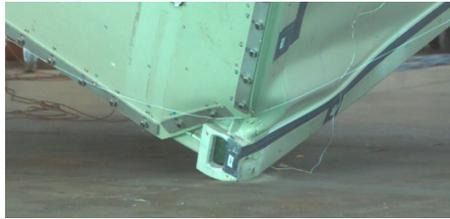
*Comparison of experiment and numerical simulation: deformation behaviour in the area of the container corner during impact*
