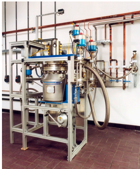
Figure 4. Cryotribometer CT3, suitable for cryogenic, vacuum and \text{H}_2 environment.
