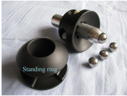
a) Test electrode and its installation
