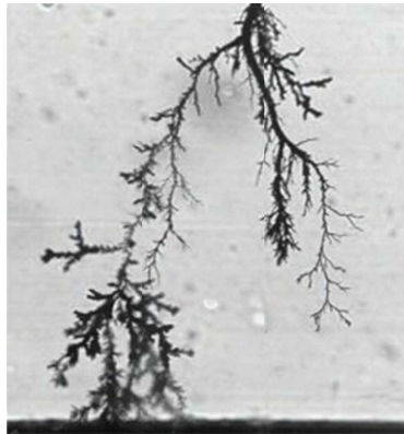
Figure 3.10: Breakdown channels in transparent polymer between point-plane electrodes
