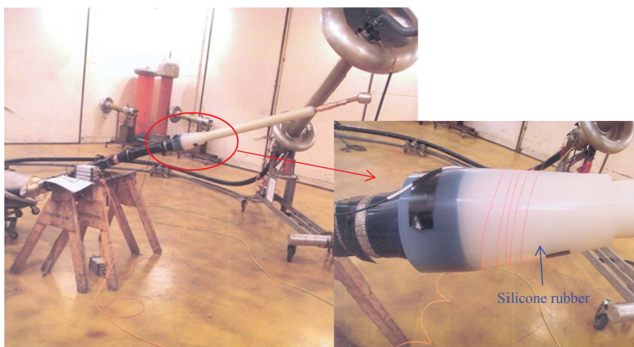
Figure 2.14: The stress-cone rubber part of HV cable accessories wrapped with the optical fibre sensor to detect PD activity inside such device [16-68]
