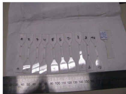
b) Specimen cured with post curing condition
