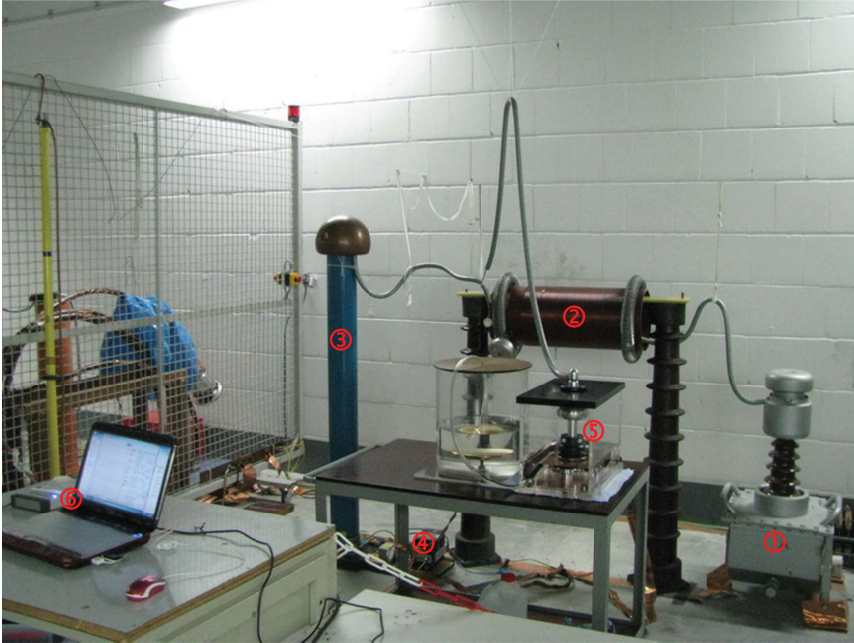
Figure 5.6: Experimental setup in the high-voltage laboratory (CESI-IPH Berlin); Notations:
