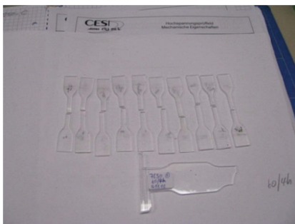
a) Specimen cured at 60 °C for 4 hours
